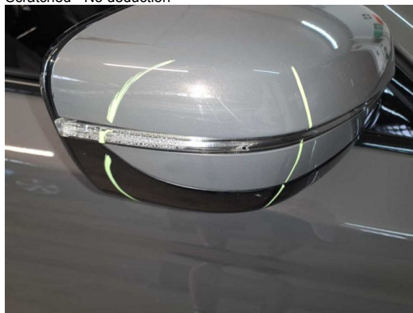
Damage #3: Indicator - front: Mirror - right side - Damaged - Replace
