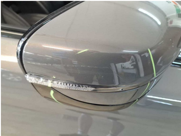
Damage #6: Wing mirror - right side: Cap - Scratched - Smart repair
