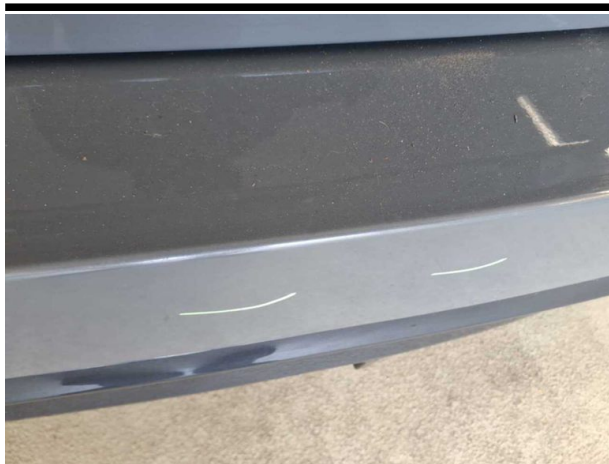
Damage #9: Rear bumper: Rear bumper - Scratched - Repair and paint
