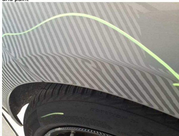
Damage #10: Side panel - rear right side: Side panel - Dent / paintcoat damage - Repair and paint
