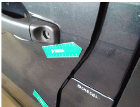
Tür / Vorne Links / Kratzer
