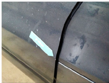
Tür / Vorne Links / Kratzer
