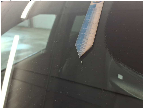
Damage 8: Vehicle glazing: Windscreen - Stone chips - Replace
