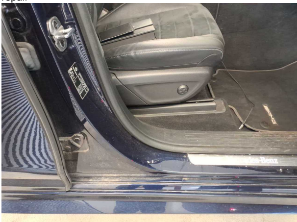
Damage 6: Sill - right side: Sill - Dent / paintcoat damage - Smart repair
