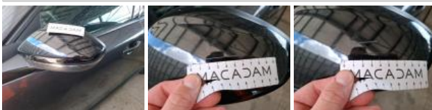
Outside rear-view mirror housing L, Scratch(es), Paint
