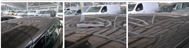
Roof, Hail damage, Repair and paint (complete)
