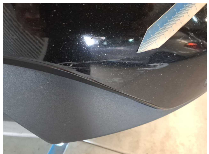
Damage 6: Front bumper: Front bumper - Scratched - Paint
