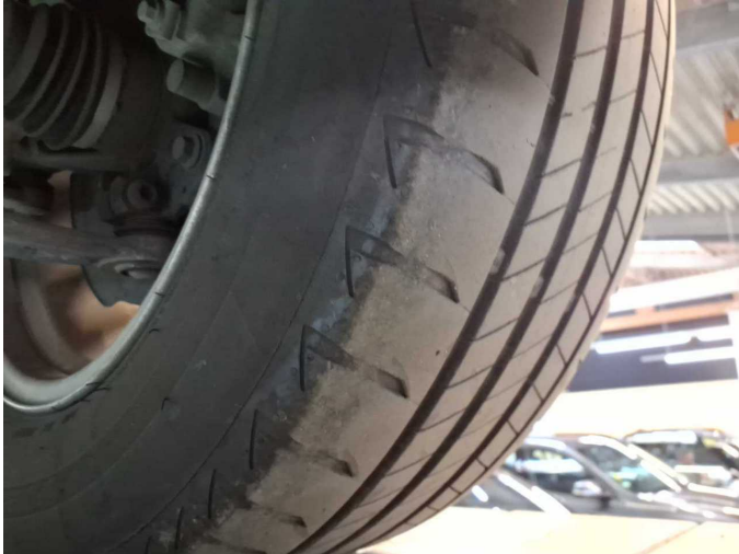
Damage 3: Front axle: Axles / undercarriage - Malposition - Measure
