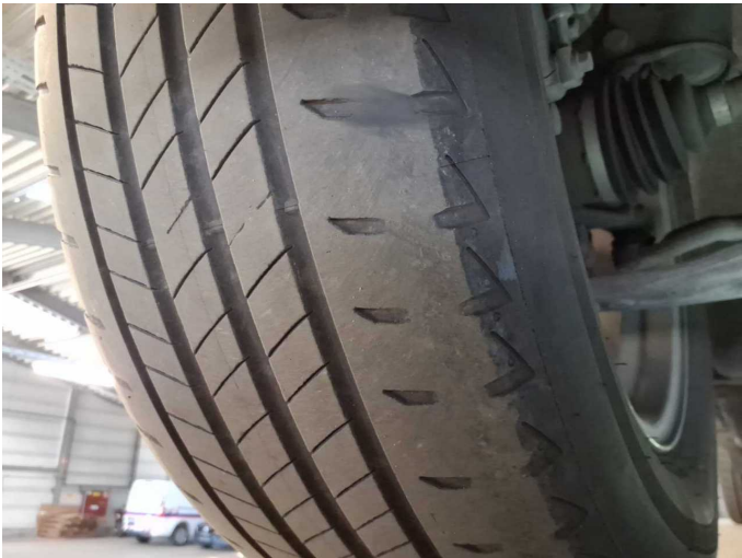
Damage 3: Front axle: Axles / undercarriage - Malposition - Measure
