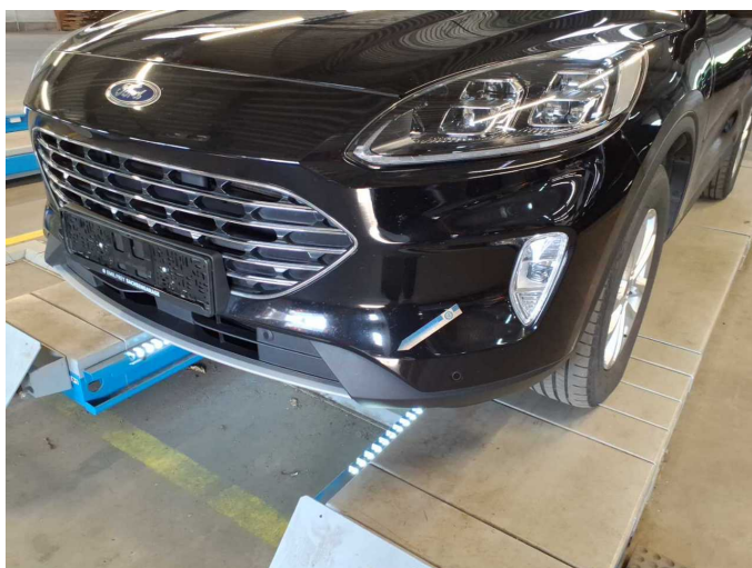
Damage 6: Front bumper: Front bumper - Scratched - Paint
