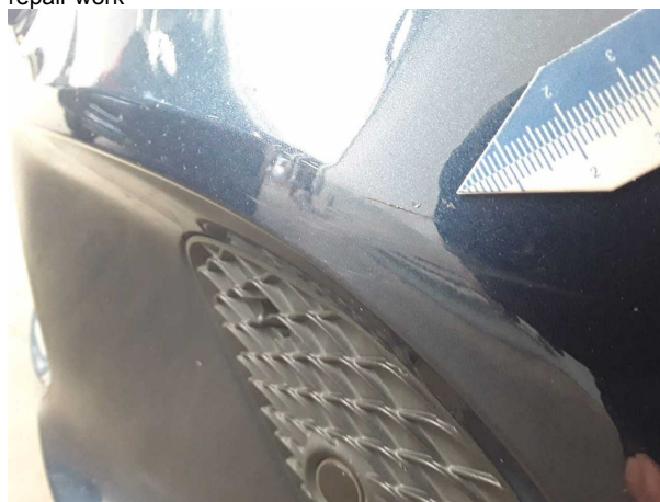
Damage #3: Front bumper: Front bumper - Scratched - Smart repair
