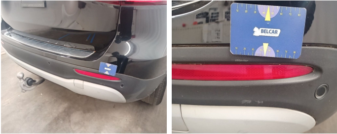
Bumper Rear / Lower Cover Not Painted / Replace-scratch
