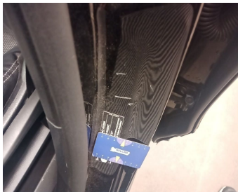
Rocker Panel Left // Smart Repair Medium-scratch + dent
