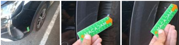
Door FL, Dent(s), Repair and paint (complete)
