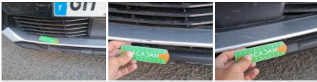
Bumper moulding F, Scratch(es), Replace
