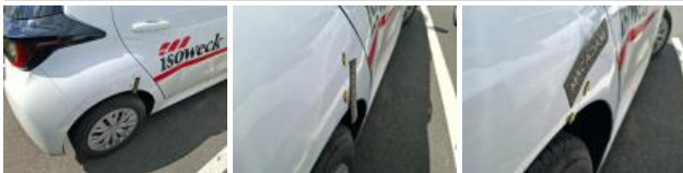
Outer sill R, Rust, Paint
