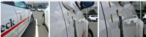
Wing RR, Bad repair, Paint
