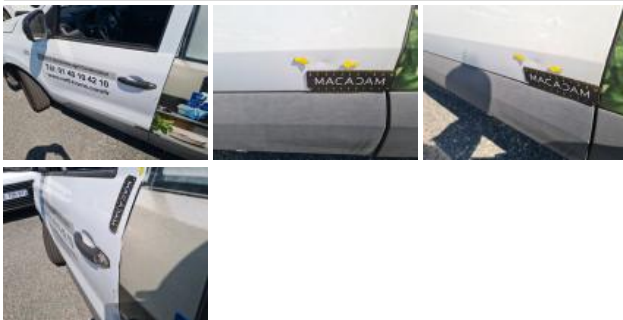
Outer door handle FL, Incomplete, Replace
