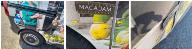
Rear light L, Broken, Replace
