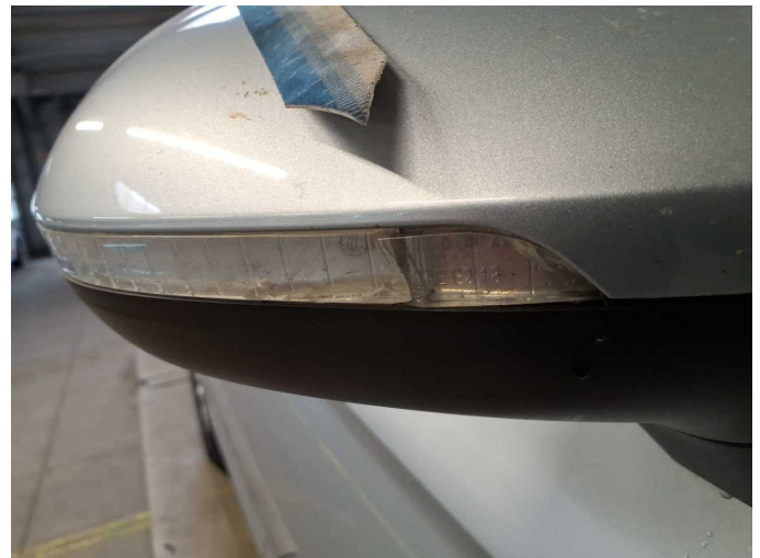
Damage 5: Indicator - front: Mirror - right side - Broken / torn - Replace
