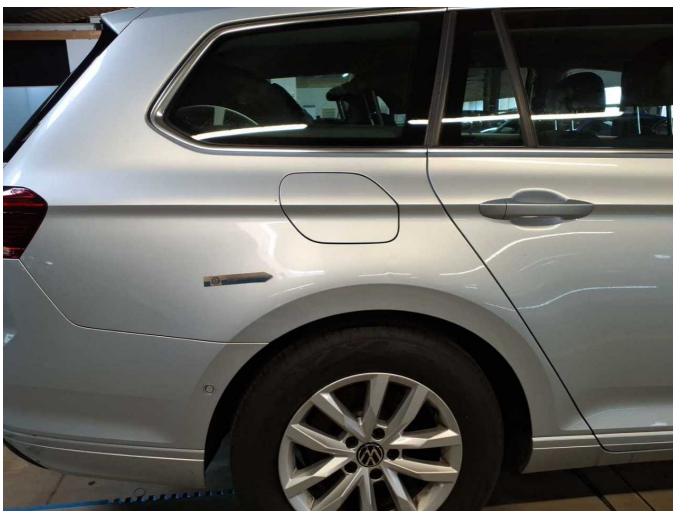
Damage 8: Side panel - rear right side: Side panel - dent(s) - Smooth repair work
