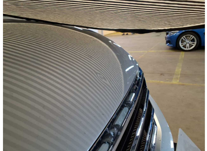
Damage 12: Bonnet: Bonnet (Wellig, wolkig, Einschlüsse) - Unprofessionally repaired - Repair and paint
