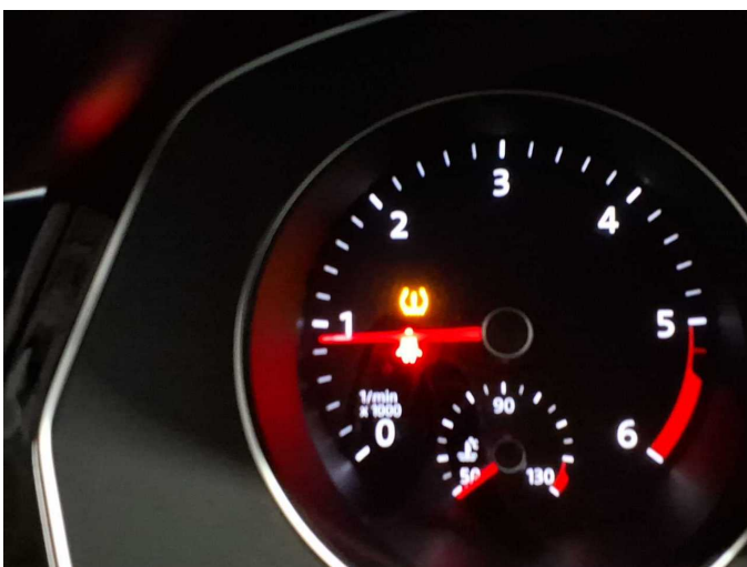
Damage 3: Wheel / tyres: Pressure sensor (Reifendruck) - Functional / admissibility - Perform diagnosis
