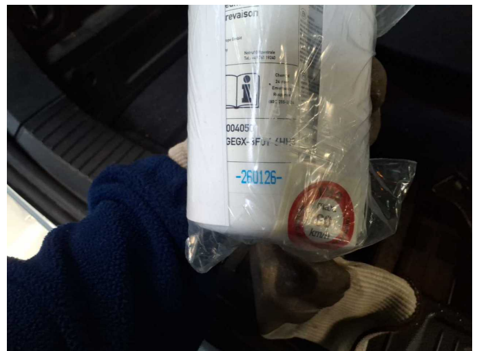
Damage 2: Equipment: Tirefit filler - Expired - Replace
