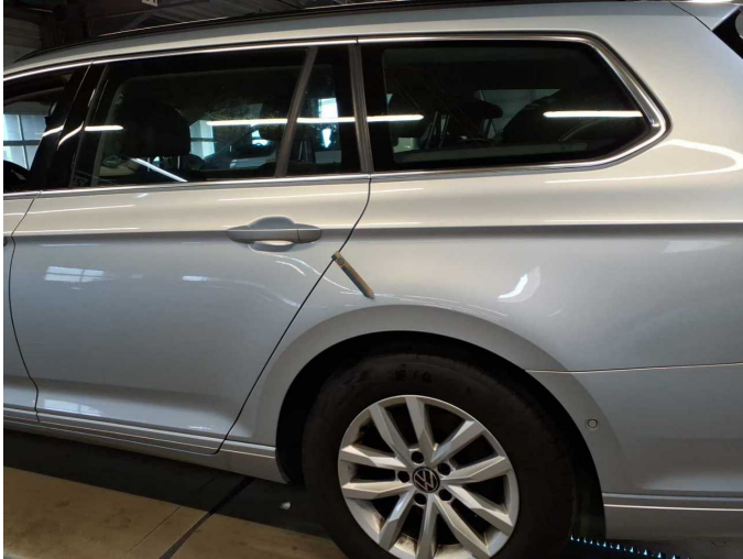
Damage 9: Side panel - rear left side: Side panel - Dent / paintcoat damage - Smart repair
