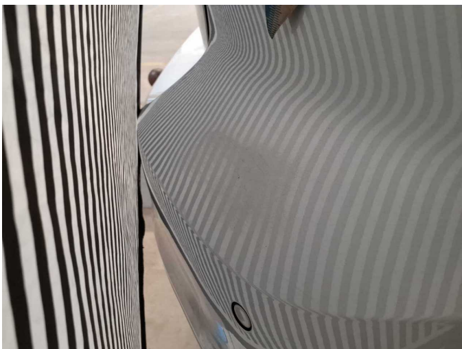
Damage 11: Rear bumper: Rear bumper (Verkratzt) - Deformed - Repair and paint
