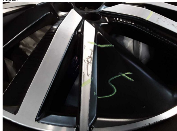
Damage #4: 2nd wheel set: 2 alloy rims - Scratched - Loss in value
