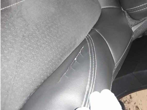
Damage #1: Seat - front: Seat cover - left side - Porous / cracked - Loss in value
