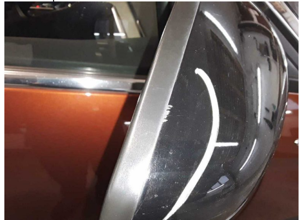
Damage #3: Wing mirror - right side: Cap - Scratched - Smart repair
