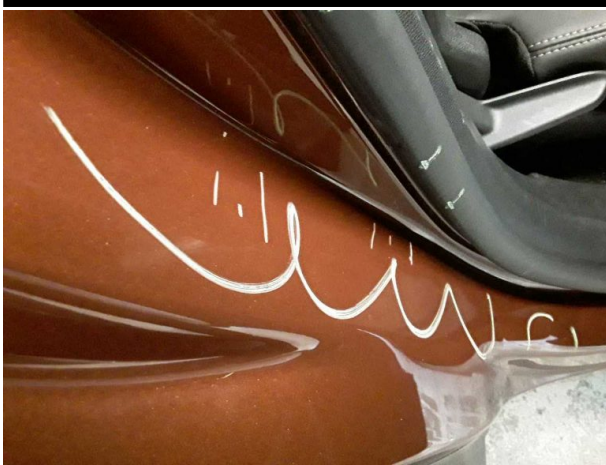
Damage #6: Side panel - rear right side: Sill - Dent / paintcoat damage - Repair and paint
