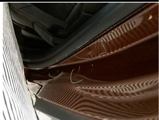
Damage #5: Side panel - rear left side: Sill - Dent / paintcoat damage - Repair and paint
