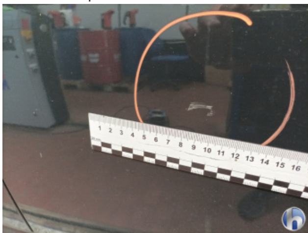
2. Tür Hinten - Links Kratzer - Smart Repair
