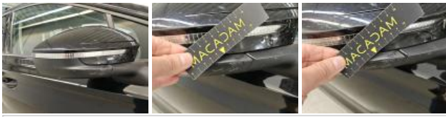
Door FR, Scratch(es), Repair and paint (complete)
