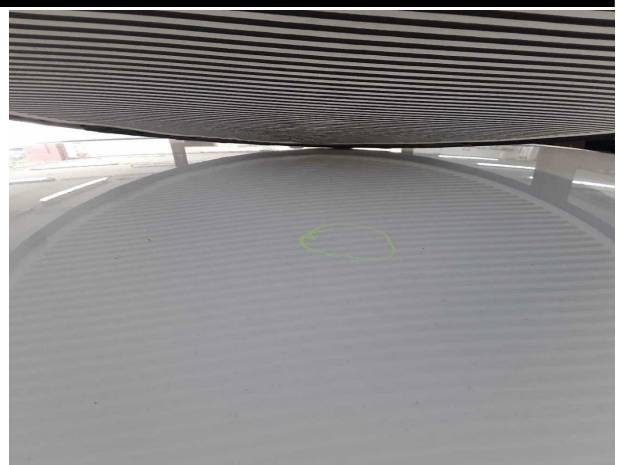
Damage #4: Roof: Roof - dent(s) - Smooth repair work
