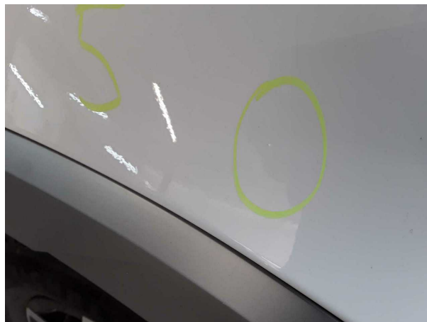
Damage #1: Side panel - rear left side: Side panel - Paint defect - Cover / polish
