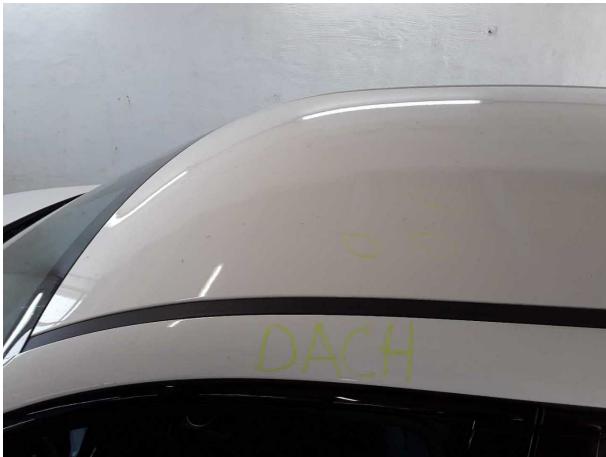
Damage #4: Roof: Roof - dent(s) - Smooth repair work
