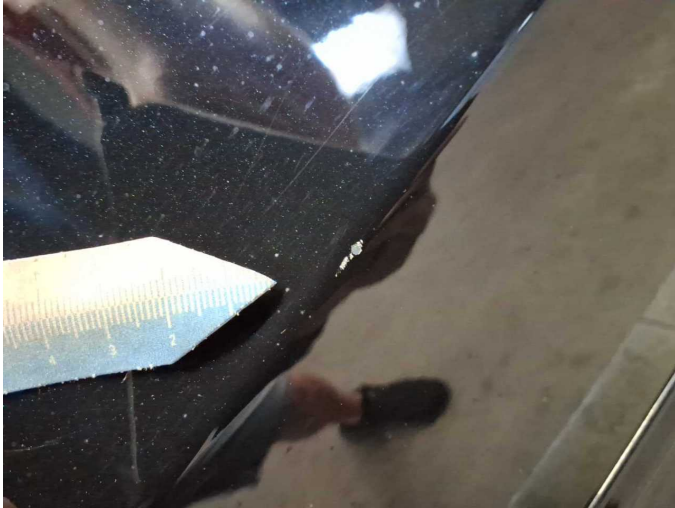
Damage 3: Door - rear left side: Door - Dent / paintcoat damage - Repair and paint
