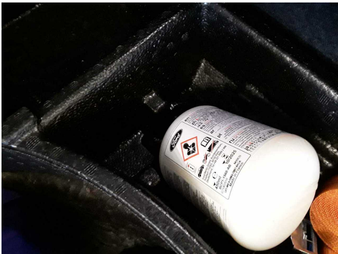
Damage 1: Equipment: Tirefit filler - Expired - Replace
