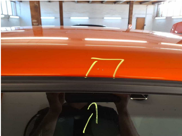
Damage #2: Roof: Roof rail - left side - Scratched - Smart repair
