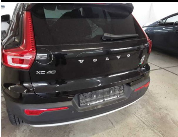
Damage #10: Boot lid / rear door: Boot lid - Dent / paintcoat damage - Repair and paint
