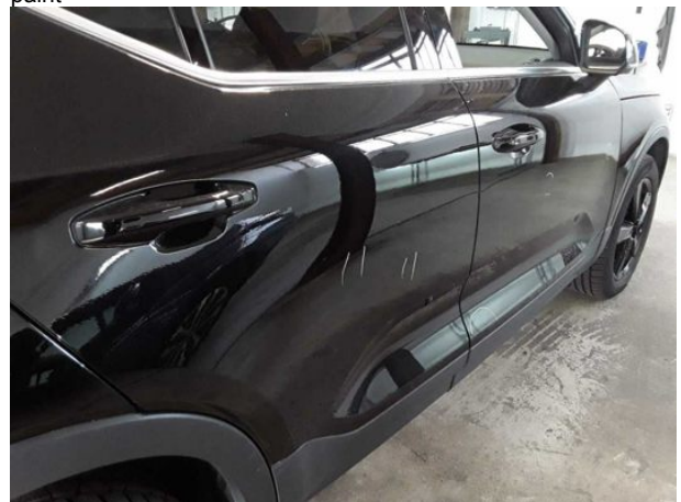
Damage #8: Door - rear right side: Door - Scratched - Repair and paint
