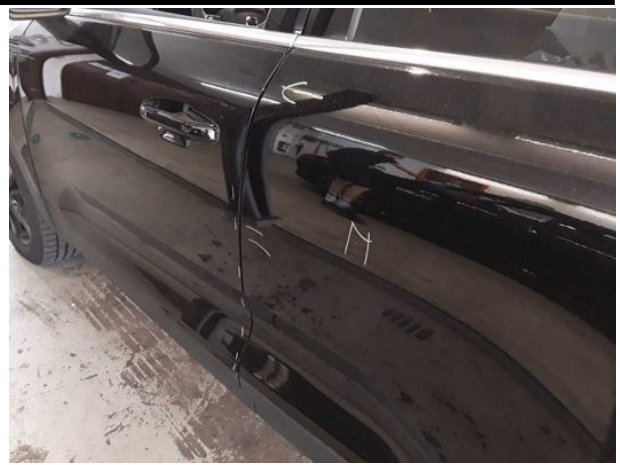
Damage #7: Door - rear left side: Door - Scratched - Repair a... paint
