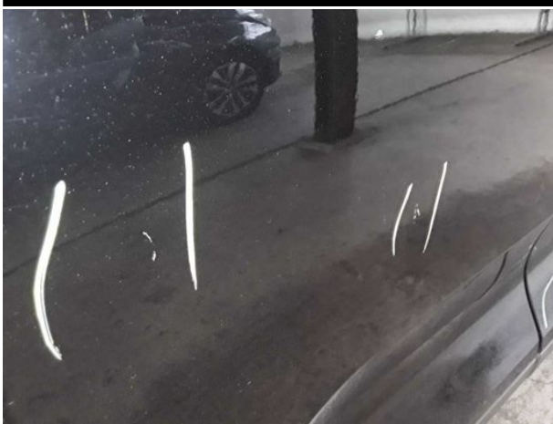
Damage #8: Door - rear right side: Door - Scratched - Repair and paint
