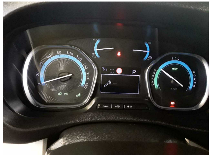
Damage 4: Misc.: Inspection / maintenance - Due - Perform
