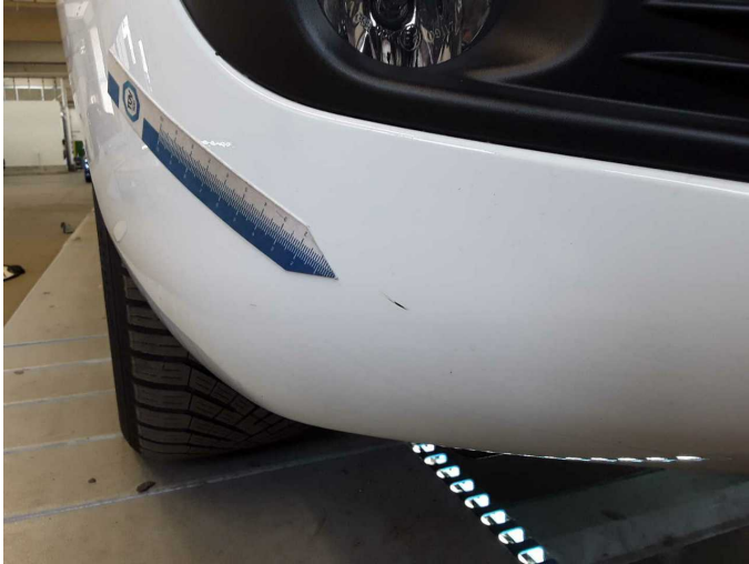
Damage 5: Front bumper: Front bumper - Scratched - Paint
