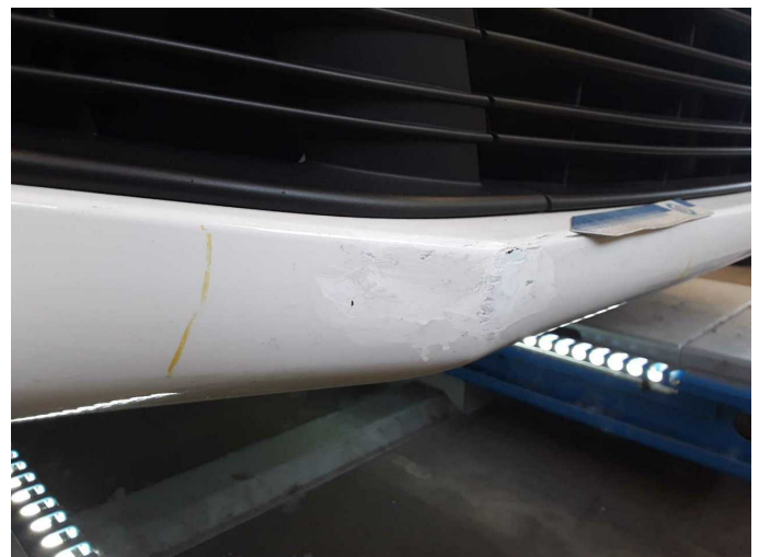
Damage 5: Front bumper: Front bumper - Scratched - Paint
