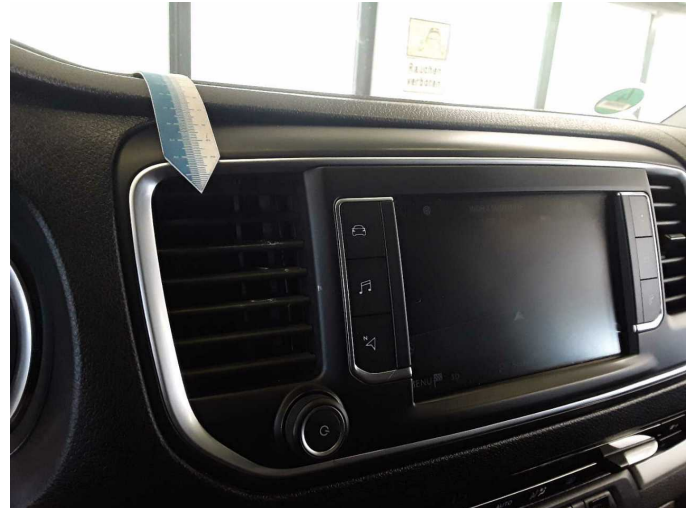
Damage 3: Instrument panel: Air nozzle - centre - Damaged - Replace
