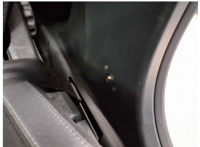
Damage 2: Trim / covers: B-pillar - trim - interior, left side (Fehlbohrungen) - Differs from the original configuration - Replace
