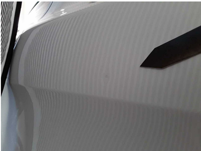
Damage 2: Mudguard - left side: Mudguard - left side - dent(s) - Smart repair
