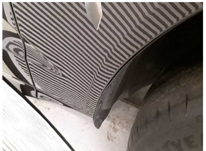
Damage 3: Mudguard - right side: Mudguard - right side - dent(s) - Paint
