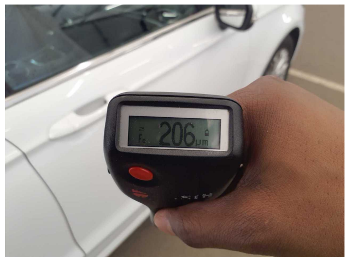
Repainting 3: Door - front right side
