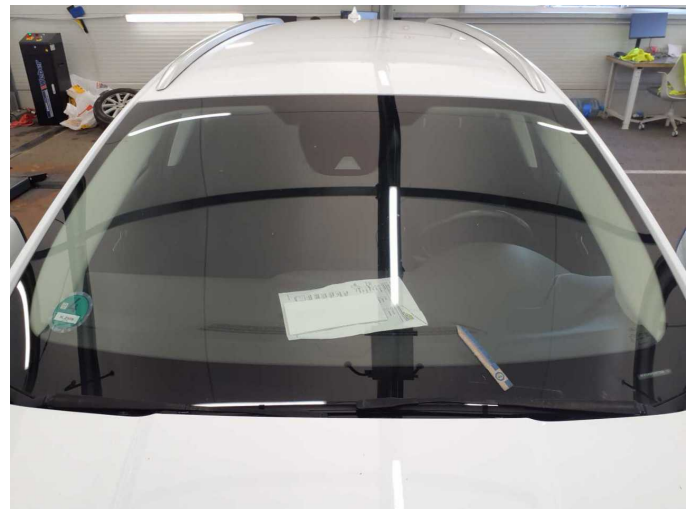
Damage 6: Vehicle glazing: Windscreen with lane departure assistant - Broken / torn - Replace
