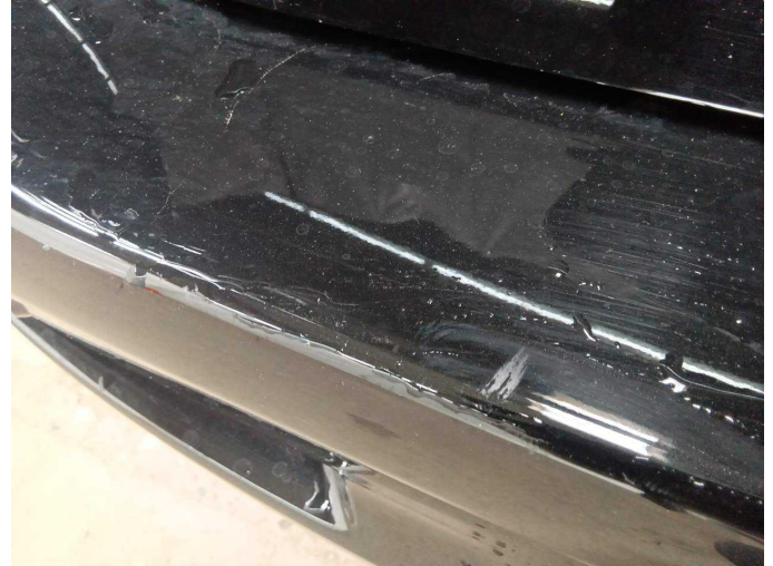
Damage 4: Rear bumper: Rear bumper - Scratch(es) - Paint
