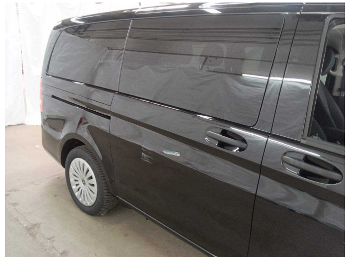
Damage 7: Sliding door, right: Sliding door - Scratched - Repair and paint
