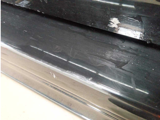
Damage 4: Rear bumper: Rear bumper - Scratch(es) - Paint
