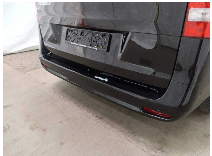
Damage 4: Rear bumper: Rear bumper - Scratch(es) - Paint
