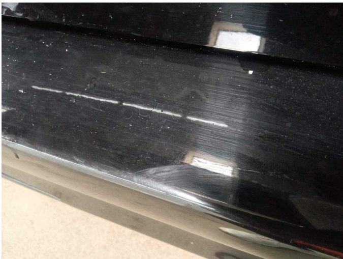
Damage 4: Rear bumper: Rear bumper - Scratch(es) - Paint
