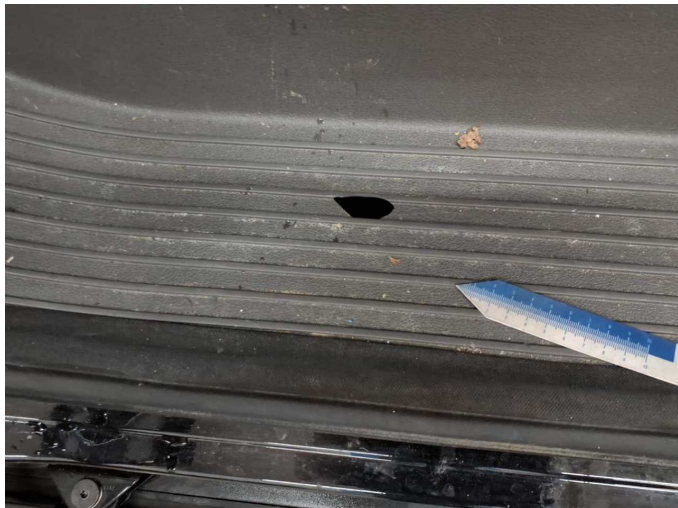
Damage 2: Trim / covers: Entrance sliding door - right side - Broken / torn - Loss in value
