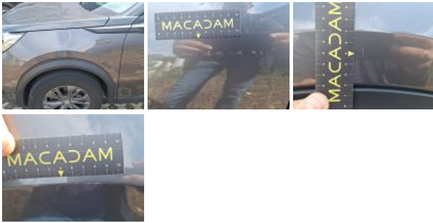
Door FL, Dent(s) and scratch(es), Acceptable
