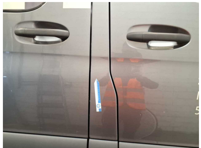
Damage 4: Body: B-pillar - right side - Scratch(es) - Smart repair
