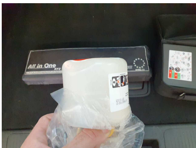
Damage 1: Equipment: Tirefit filler - Empty - Replace
