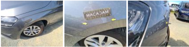
Wing RL, Dent(s) and scratch(es), Repair and paint (complete)
