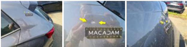
Door RL, Dent(s) and scratch(es), Repair and paint (complete)
