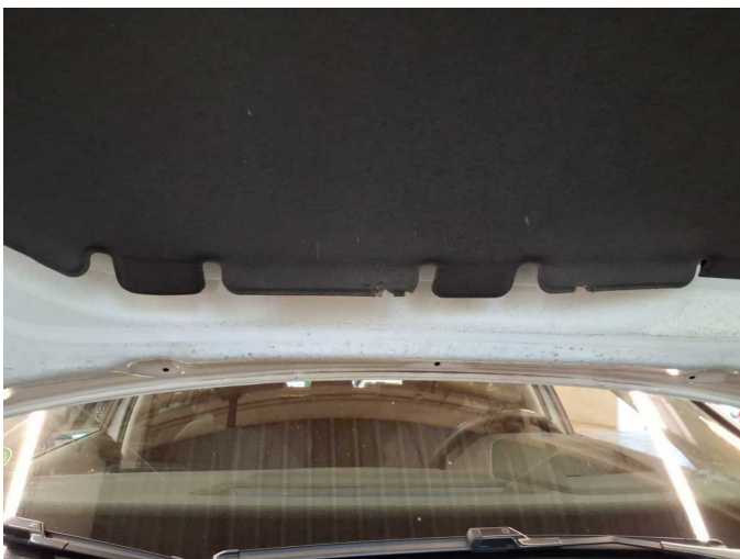
Damage 4: Bonnet: Insulation lining - Broken / torn - Replace
