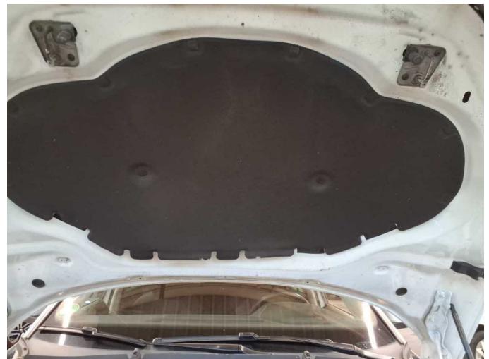
Damage 4: Bonnet: Insulation lining - Broken / torn - Replace
