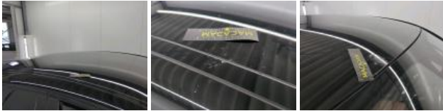
Roof, Chemical polution, Repair and paint (complete)
