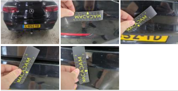
Bumper moulding RL, Scratch(es), Replace and paint
