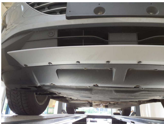
Damage 6: Front bumper: Spoiler - Scratch(es) - Replace
