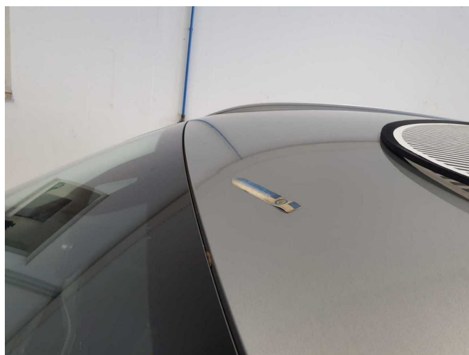
Damage 4: Roof: Roof - dent(s) - Smooth repair work
