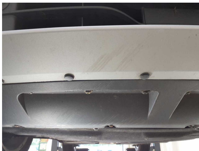
Damage 6: Front bumper: Spoiler - Scratch(es) - Replace
