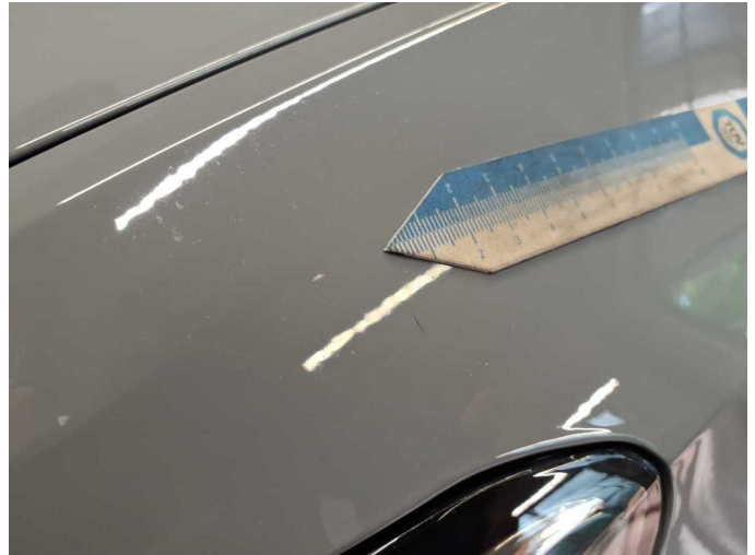
Wear and tear 2: Mudguard - left side: Mudguard - left side - Stone chips - No deduction
