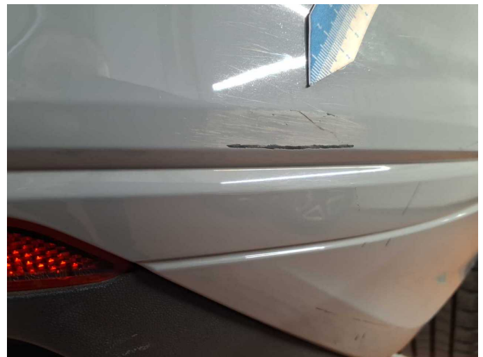
Damage 4: Rear bumper: Rear bumper - Scratched - Paint
