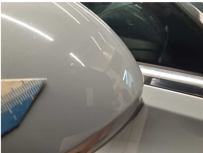
Wear and tear 3: Wing mirror - right side: Cap - Stone chips - No deduction
