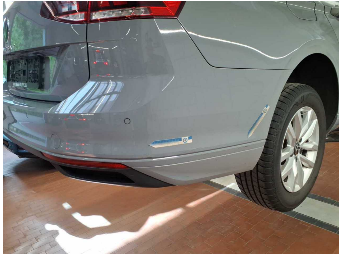
Damage 4: Rear bumper: Rear bumper - Scratched - Paint
