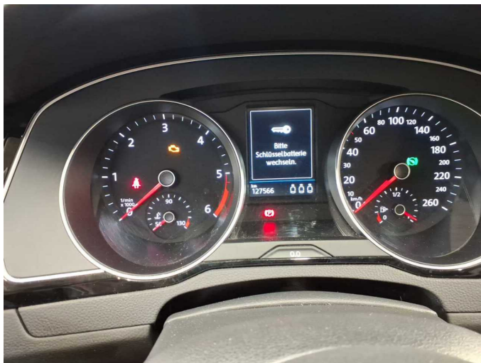
Damage 1: Equipment: Vehicle key with remote control (Batterie erneuern) - Non-operational - Replace
