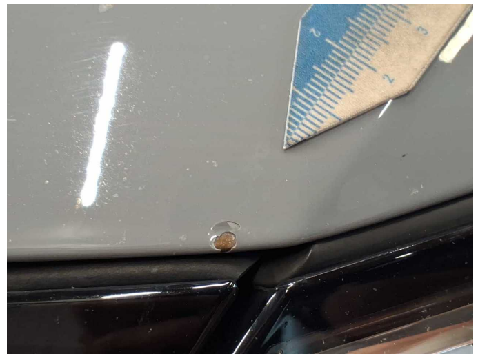
Damage 5: Bonnet: Bonnet - Corrosion - Paint
