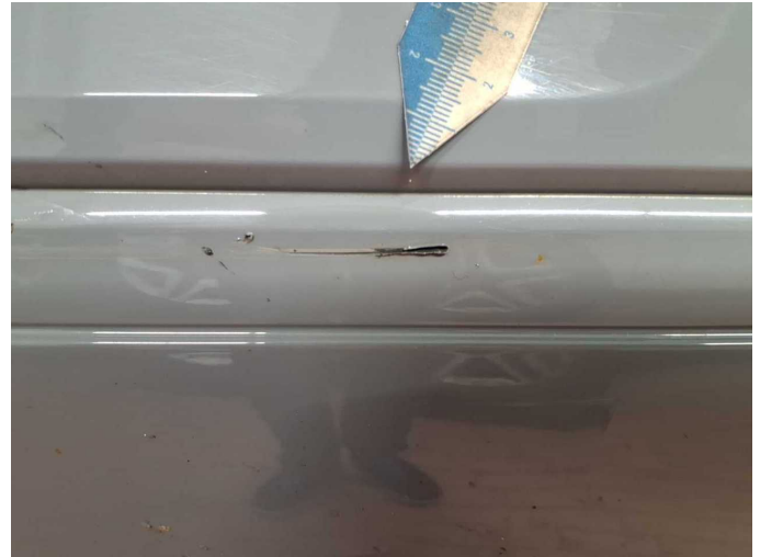
Damage 4: Rear bumper: Rear bumper - Scratched - Paint
