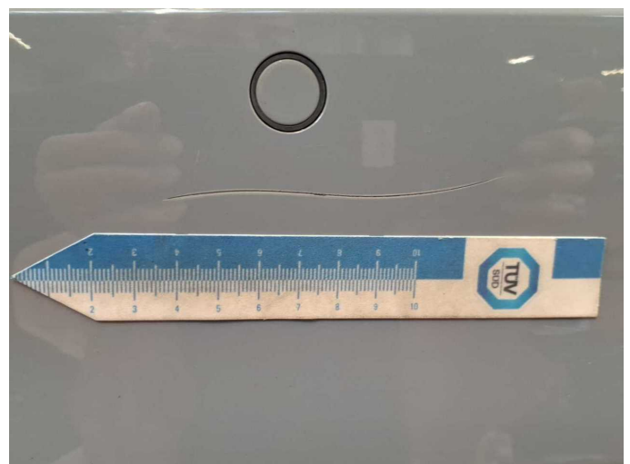
Damage 4: Rear bumper: Rear bumper - Scratched - Paint
