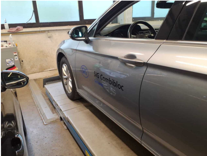
Damage 1: Body: Body - Glued / labelled - De-glue / neutralise
