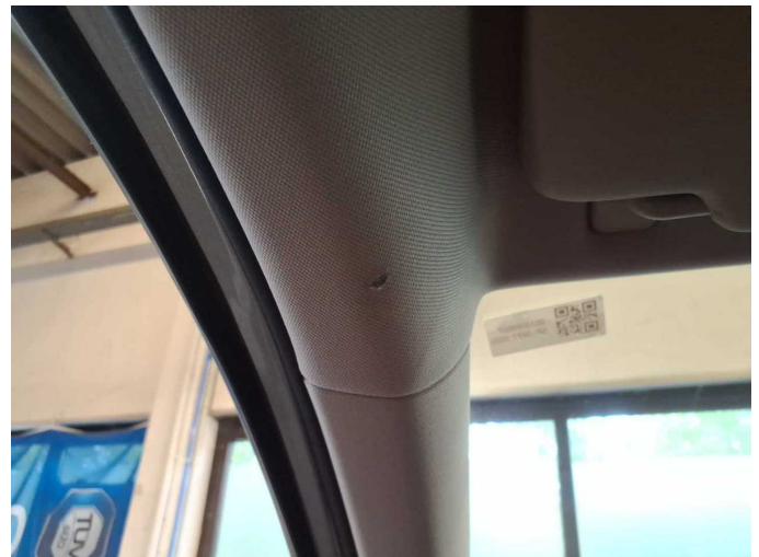
Damage 4: Trim / covers: Roof lining (Vorne Links) - Burn hole (cigarettes) - Smart repair
