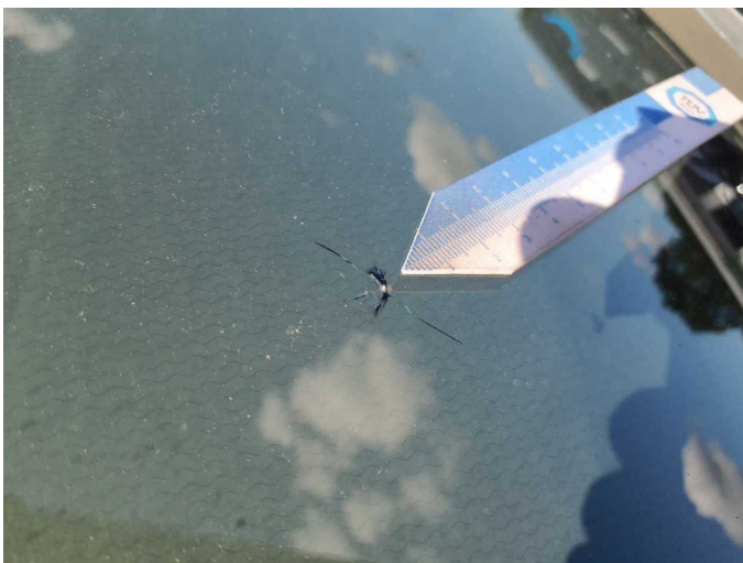
Damage 4: Vehicle glazing: Windscreen - Broken / torn - Replace
