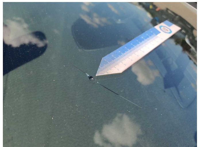
Damage 4: Vehicle glazing: Windscreen - Broken / torn - Replace
