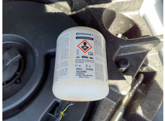
Damage 2: Equipment: Tirefit filler - Expired - Replace
