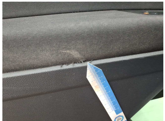
Damage 12: Trim / covers: Door trim - front right side - Broken / torn - Replace
