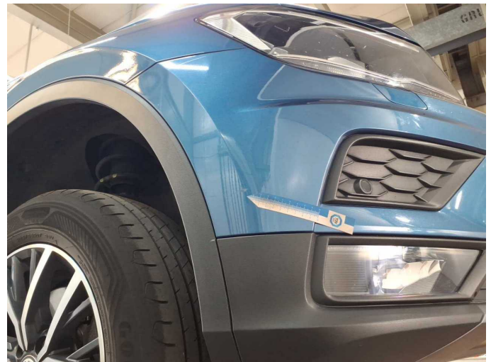
Damage 19: Front bumper: Front bumper - Scratch(es) - Paint
