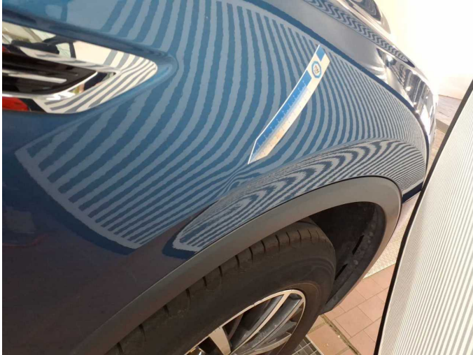
Damage 8: Mudguard - right side: Mudguard - right side - dent(s) - Smart repair
