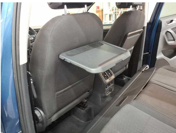
Damage 5: Equipment: Table support - Non-operational - Replace
