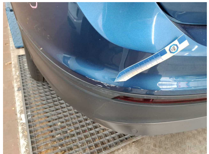
Damage 16: Rear bumper: Rear bumper - Scratch(es) - Paint
