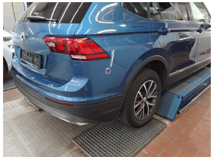
Damage 16: Rear bumper: Rear bumper - Scratch(es) - Paint
