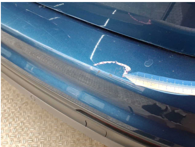
Damage 16: Rear bumper: Rear bumper - Scratch(es) - Paint
