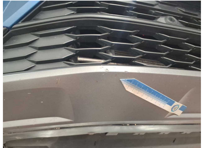
Damage 11: Front bumper: Spoiler - Scratch(es) - Paint
