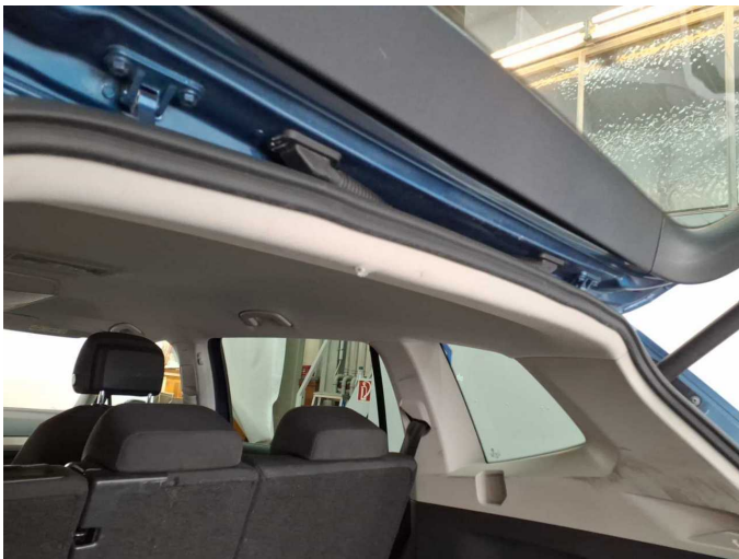
Damage 15: Trim / covers: Roof lining - Broken / torn - Replace
