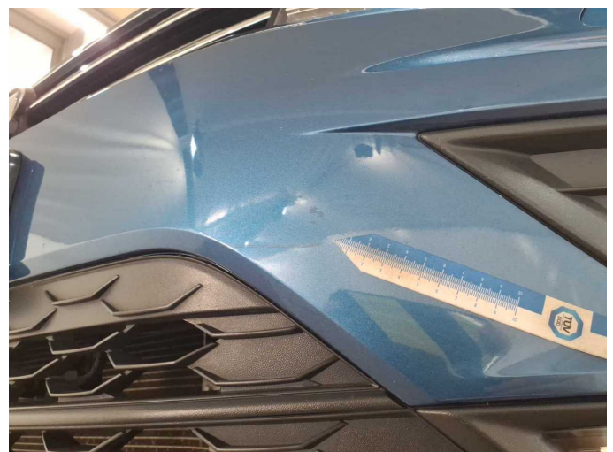
Damage 19: Front bumper: Front bumper - Scratch(es) - Paint
