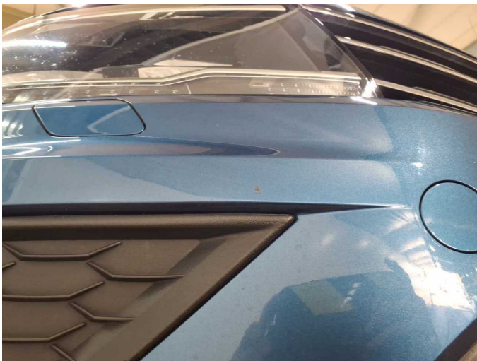
Damage 19: Front bumper: Front bumper - Scratch(es) - Paint
