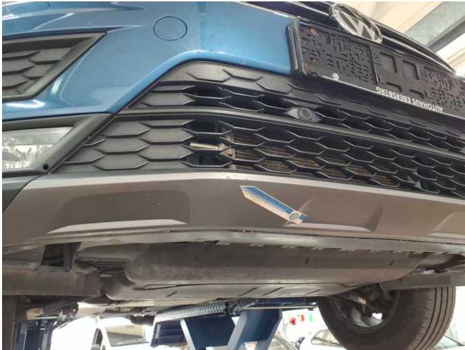
Damage 11: Front bumper: Spoiler - Scratch(es) - Paint
