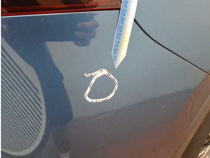
Damage 16: Rear bumper: Rear bumper - Scratch(es) - Paint
