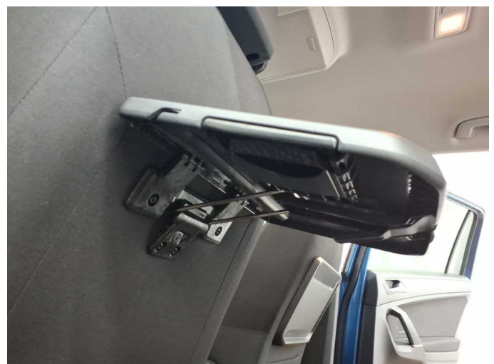
Damage 5: Equipment: Table support - Non-operational - Replace
