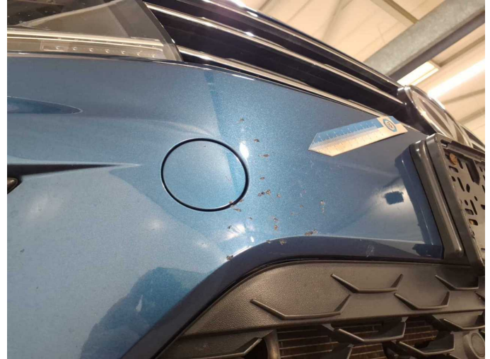
Damage 19: Front bumper: Front bumper - Scratch(es) - Paint
