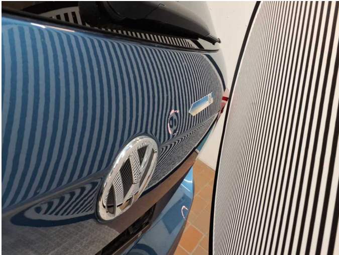
Damage 21: Boot lid / rear door: Boot lid - dent(s) - Repair and paint
