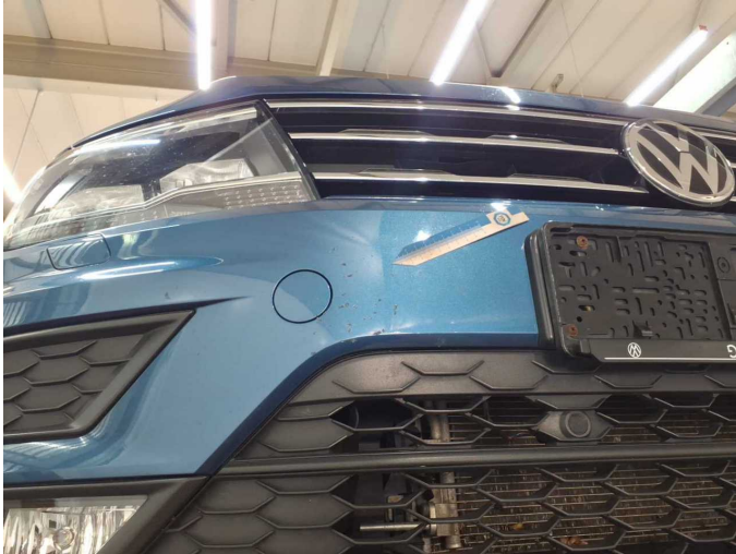
Damage 19: Front bumper: Front bumper - Scratch(es) - Paint
