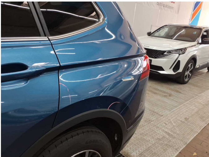
Wear and tear 8: Side panel - rear left side: Side panel - dent(s) - Repair and paint
