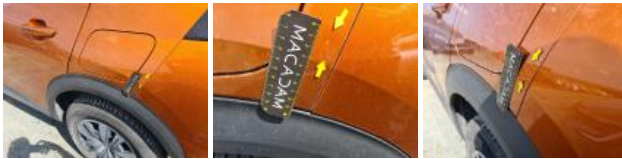
Door RL, Scratch(es), Paint
