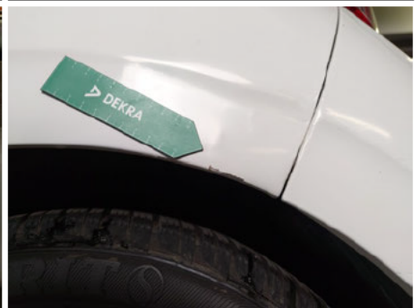
Kotflügel / Hinten Links / Delle
