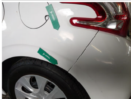
Kotflügel / Hinten Links / Delle
