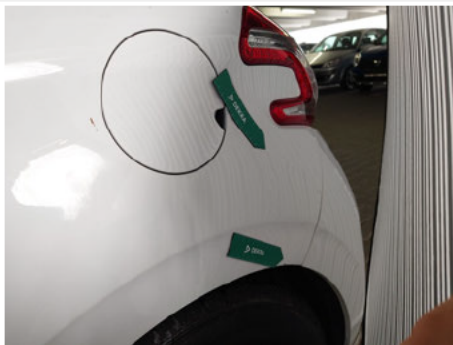
Kotflügel / Hinten Links / Delle
