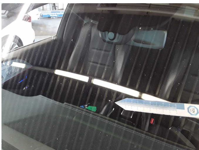
Damage 2: Vehicle glazing: Windscreen - Stone chips - Replace
