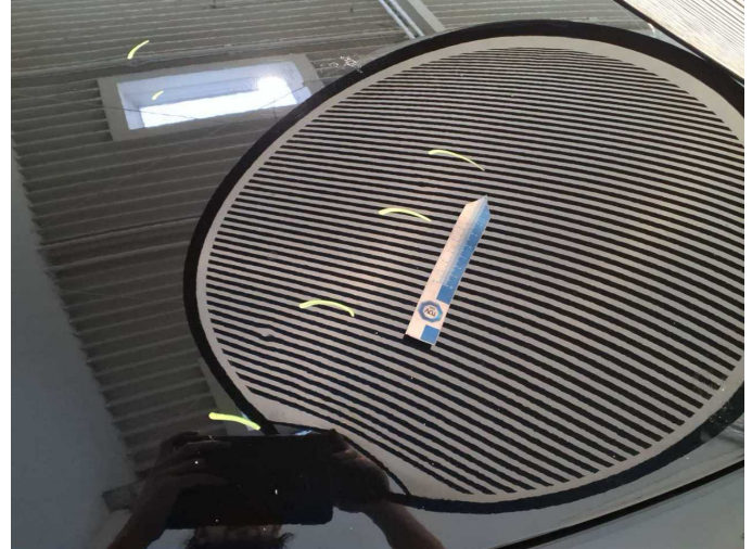
Damage 4: Body: Body - Damage by hail - Smooth repair work
