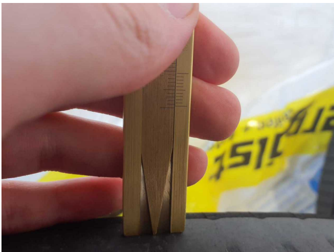
Damage 8: 2nd wheel set: 2 tyres - Worn - Replace
