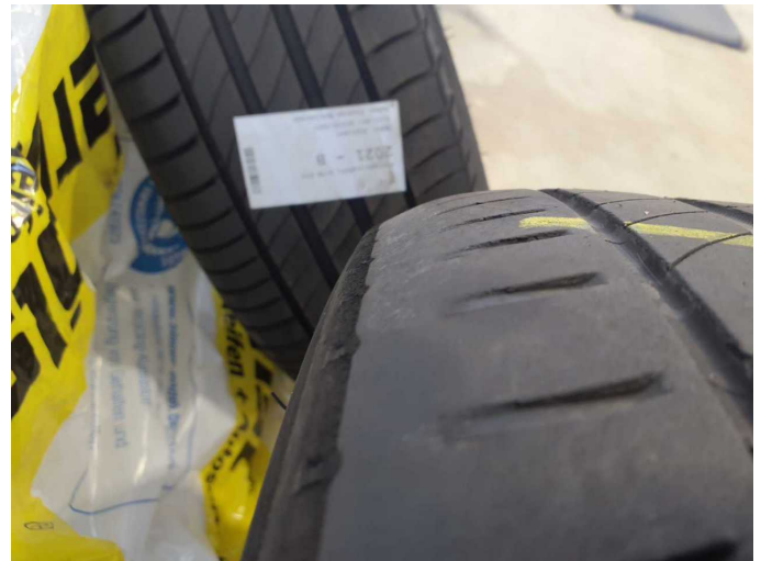
Damage 8: 2nd wheel set: 2 tyres - Worn - Replace
