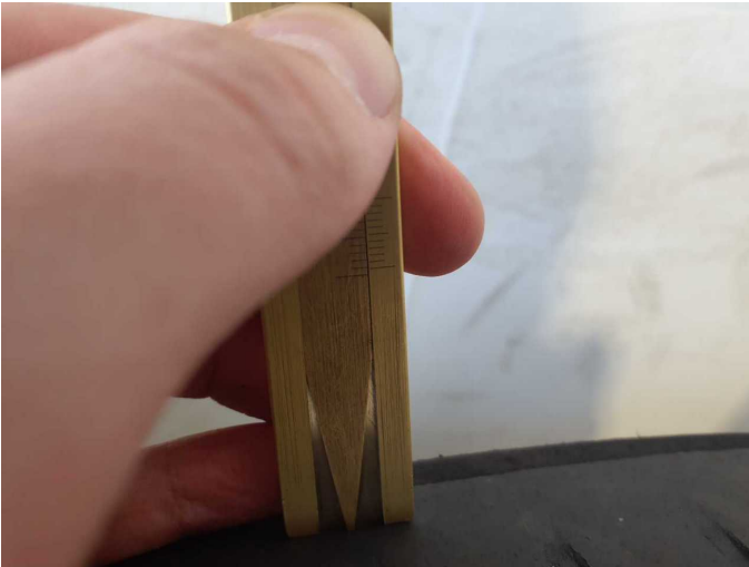
Damage 8: 2nd wheel set: 2 tyres - Worn - Replace
