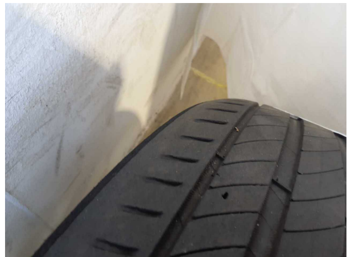
Damage 8: 2nd wheel set: 2 tyres - Worn - Replace
