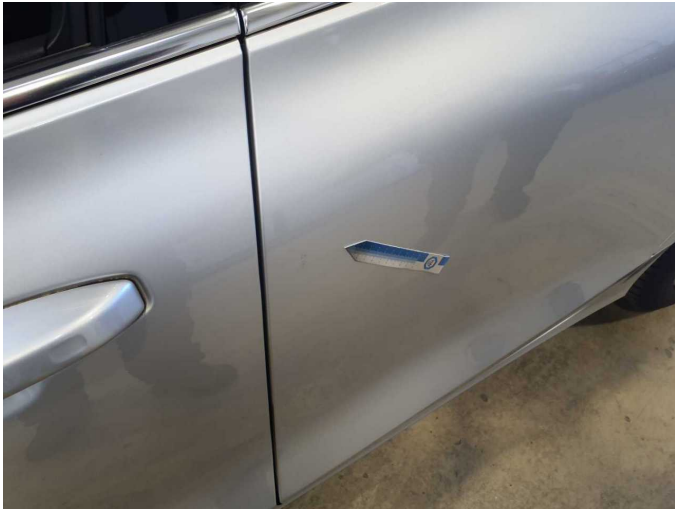
Damage 4: Door - rear left side: Door - Dent / paintcoat damage - Smart repair
