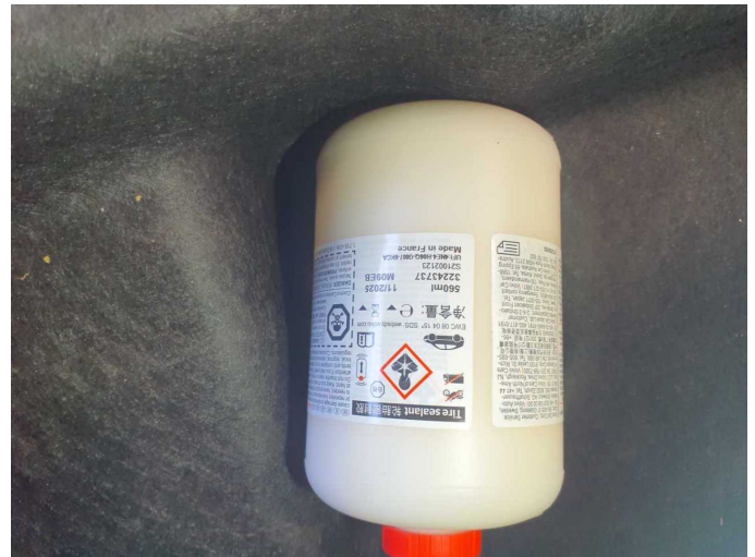
Damage 2: Equipment: Tirefit filler - Expired - Replace
