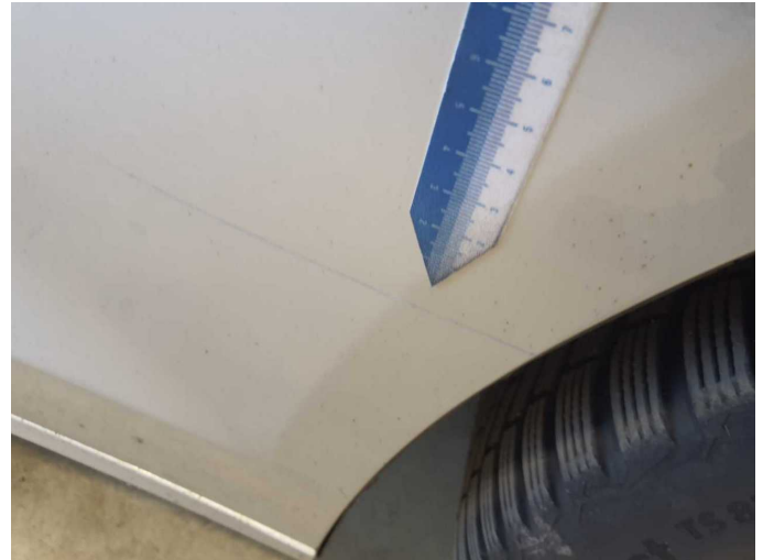
Damage 11: Mudguard - right side: Mudguard - right side - Dent / paintcoat damage - Repair and paint
