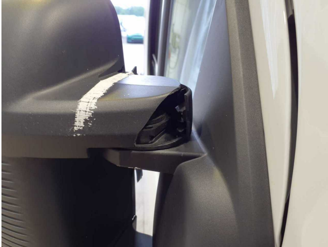
Damage 3: Wing mirror - right side: Mirror housing - Broken / torn - Replace
