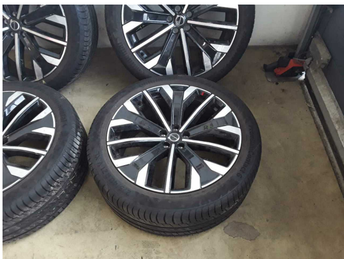
Damage 5: 2nd wheel set: 1 alloy rim (Materialabtrag) - Scratched - repair according to calculation
