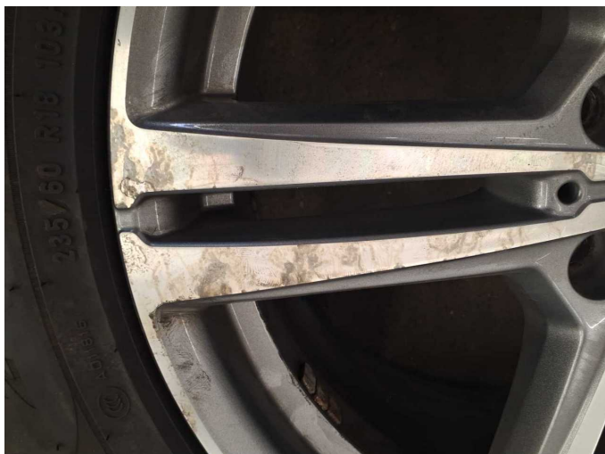
Damage 1: 2nd wheel set: 1 alloy rim (Klarlack löst sich) - Paint defect - Loss in value
