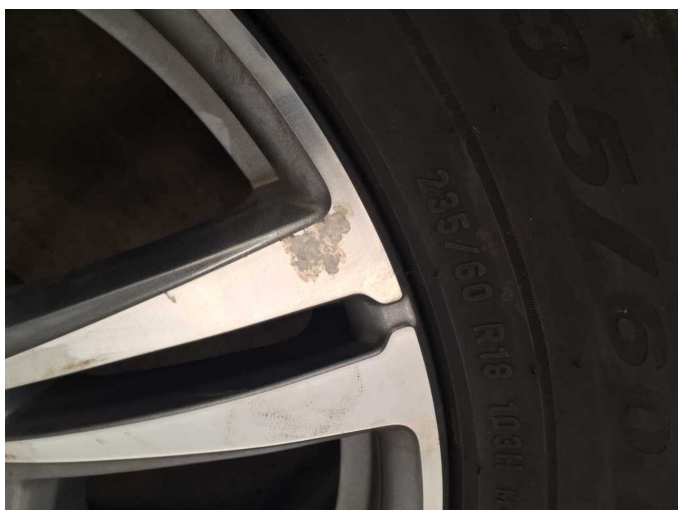
Damage 2: 2nd wheel set: 1 alloy rim (Klarlack löst sich) - Paint defect - Loss in value
