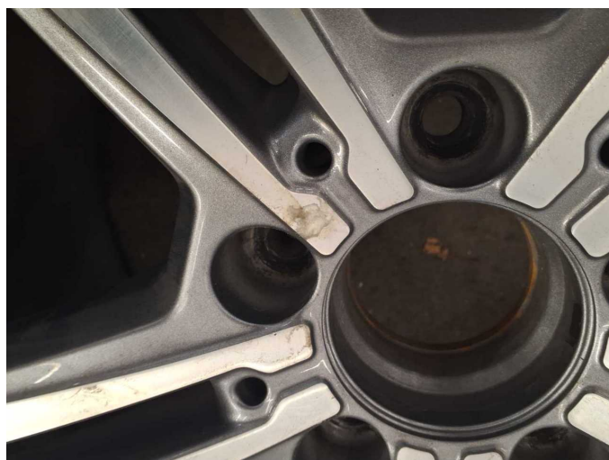
Damage 3: 2nd wheel set: 1 alloy rim (Klarlack löst sich) - Paint defect - Loss in value
