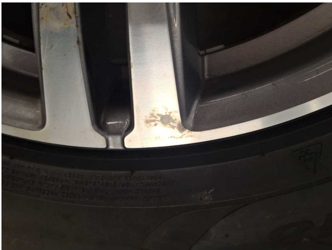
Damage 4: 2nd wheel set: 1 alloy rim (Klarlack löst sich) - Paint defect - Loss in value
