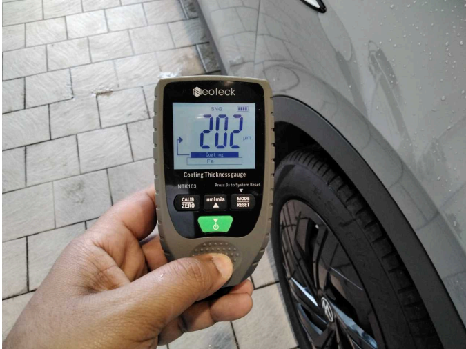
Mudguard - right side: 202 µm
