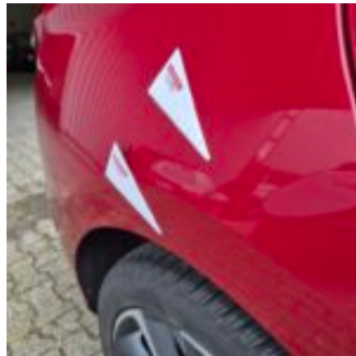
Damage Type Small dent(s)
