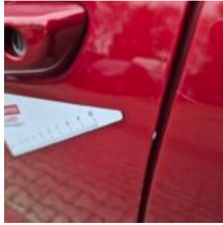
Damage Type Door-edge chipped
