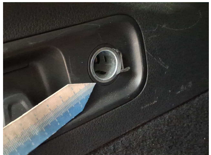
Damage 2: Interior: Cigarette lighter (im Kofferraum) - Broken / torn - Replace
