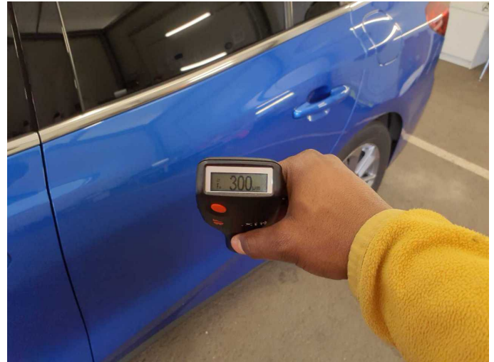
Repainting 4: Door - rear left side
