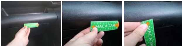
Glove compartment lid, Scratch(es), Replace
